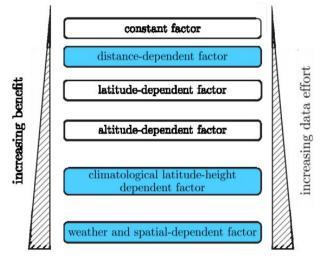
Figure 1 - Schematic overview of different possible abstraction levels to estimate aviation non-CO<sub>2</sub> effects
